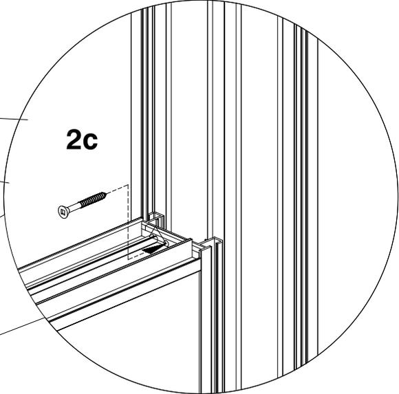
2c. Install Securing Screw(s).
