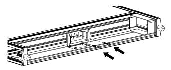
Attach required duplex receptacles to the power block.
