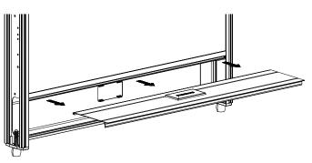
4. Drill marked holes with  $\frac{1}{8}$ " drill bit.
