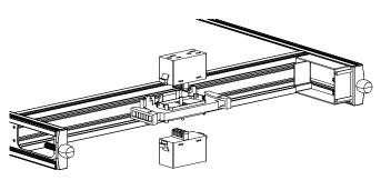
Remove grommet cover and push raceway cover straight in to attach.
